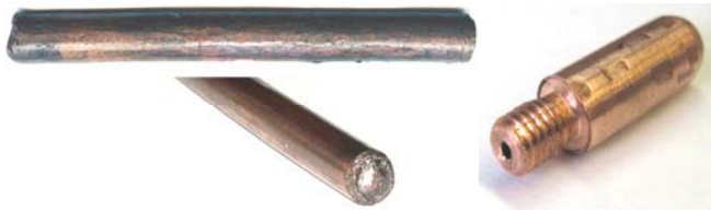
Fig. 3. The details produced from fibrous copper
