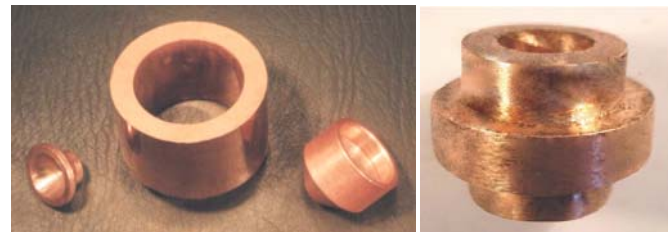
Fig. 2. Details made of copper powder produced from wastes of copper current conductors
