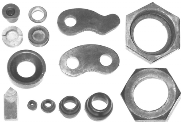
Fig. 4. The details produced from structural heterogeneous iron-based powder materials
