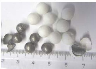
Fig. 2 Iron hollow balls (kaolin coated and non-coated)
