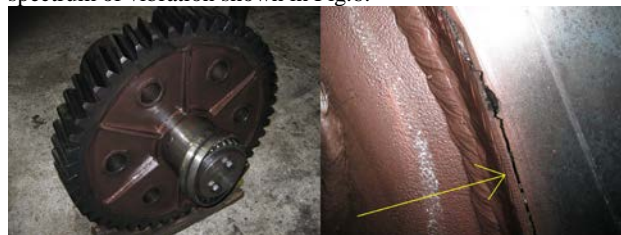
Figure 6. The photo of the real welded gearwheel, with the cracks. As can be seen, due to this method, was sufficiently prevented a serious accident and were spared a lot of resources.
