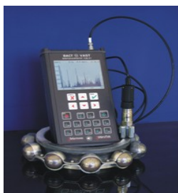
Figure 2. Vibration portable set on the vibration analyzer CD-21 base, produced by company BACT (Russia) [2]
