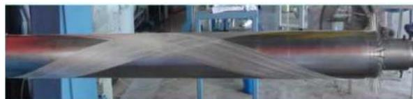
low winding angle ( $\theta = 10^\circ$ )
