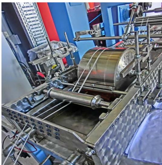
Figure 2. Filament winding machine MAW FB 6/1
