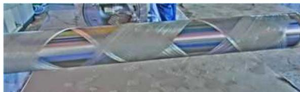
helical winding ( $\theta = 45^\circ$ )
