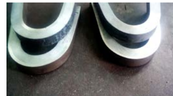
Figure 3 Bend specimens after testing
