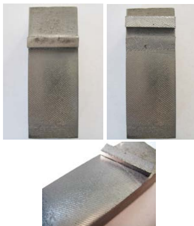
Figure 6 Specimen for shear test before and after testing
