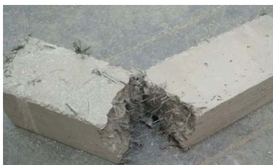
Fig 4 Beam specimen after 3 point flexure test
