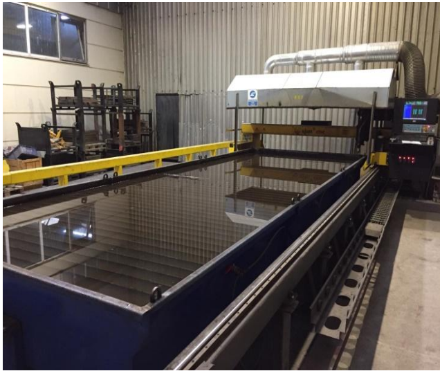
Fig. 2. AJAN CNC 2x6m PP260A plasma cutting
