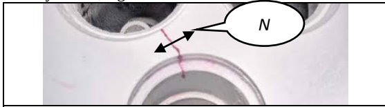
Fig.3. Semi-elliptical crack between cylinders in the diesel engine
