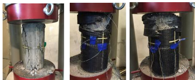
Fig. 5 - Photo of the destroyed samples without amplification, with 1st and 3rd gain grids
