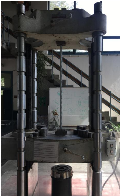
Figure 2: Experimental Setup, Force controlled test machine
