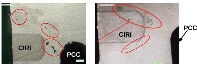
Fig. 4. Macrostructures of an improper insert-piston joint: (a) shrinkage cavities between the insert (CIRI) and the piston cooling channel (PCC); (b) porosity around the insert (property of Federal-Mogul Gorzyce sp. z o.o.).
