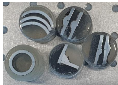
Fig. 2. Samples prepared for optical microstructural analysis: pipe parts and welds
