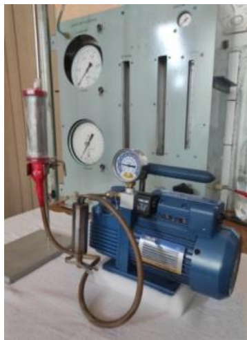
Fig. 9. Testing the filter element for its ability to withstand a given pressure drop (up to 1 bar).
