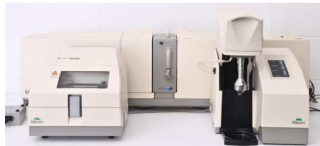
Fig. 4. Mastersizer 2000 laser diffraction particle size analyzer with HydroS automatic sample dispersion and feed module (Malvern Instruments Ltd., UK).
