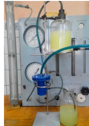
Fig. 3. Device for determining the filtration fineness of liquid during the filtration process.
