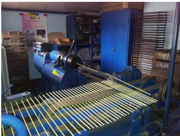
Fig.3 . Manufacturing line rods WRAPPED for brazing .
