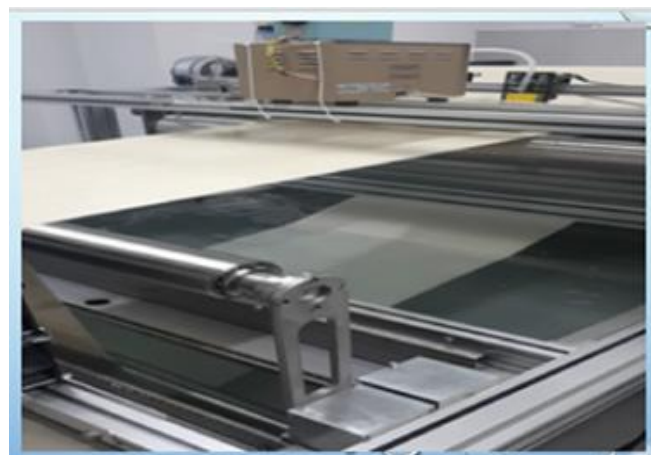
Fig.2 110 cm wide membrane production device
