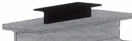
Figure 9 T - shape connector
