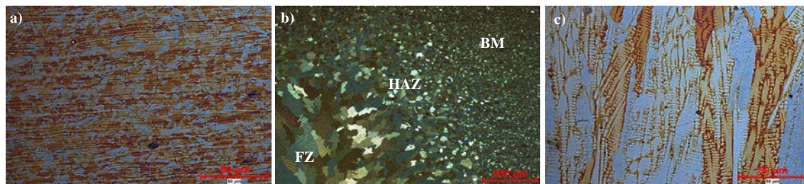
Fig.2 Microstructural changes from the BM to the FZ via optical microscopy observations. (a) BM, (b) transition zone between FZ and BM, (c) FZ. (The joint with welding time of 300 ms).
