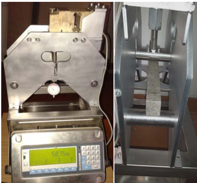
Fig.6. Experimental setting for determining the static modulus
