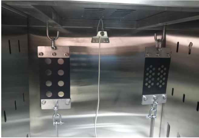
Fig. 4 Installment of the samples in the chamber
