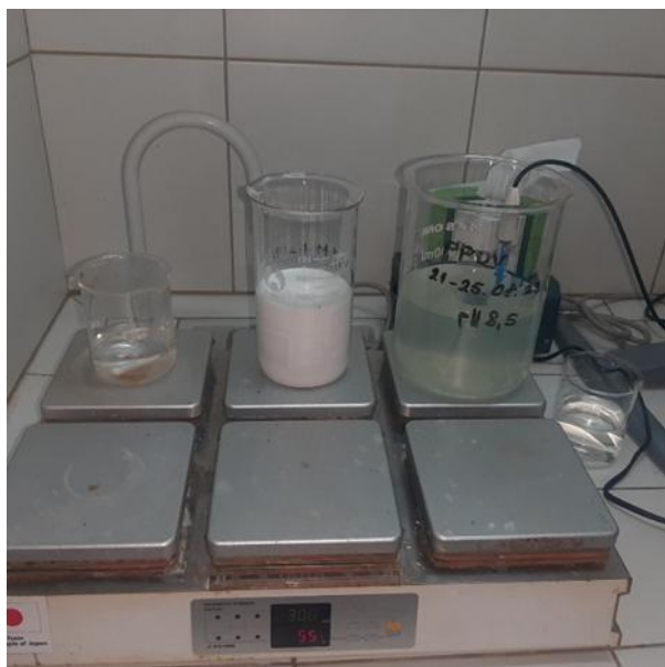
Figure 1. Neutralization of flowing water to pH8.5
