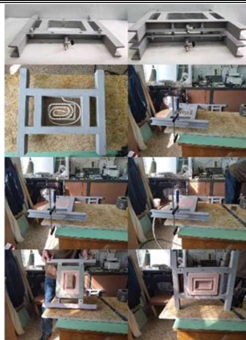
Fig. 5. Technological process in the production of a matrix structure for pressing ceramic products – reduced paving stones from semi-dry modified marl clay.
