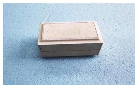
Fig. 3. Gypsum model of a reduced block for outdoor flooring on a scale of 1:2 compared to the original paving block - yellow paving stone.
